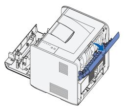
3 Open the side cover by pressing the two detents on the front right side of the machine and swinging the cover back.
